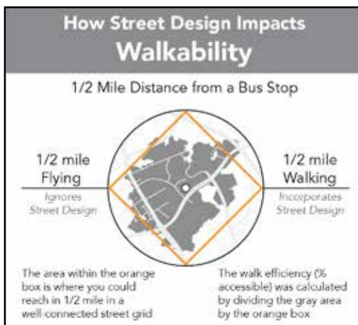
Figure 27: Walkability looks at how street design impacts how far someone can walk in a limited amount of time. A highly gridded interconnected road network will allow someone to travel farther in a short walk than a disconnected area with limited street access.
