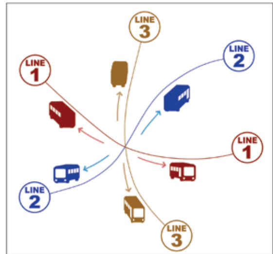
Figure 21: This graphic helps show how a pulse (or timed connection) allows a rider to transfer between multiple routes with a single timed transfer. This multiplies the amount of total destinations available to a rider.
